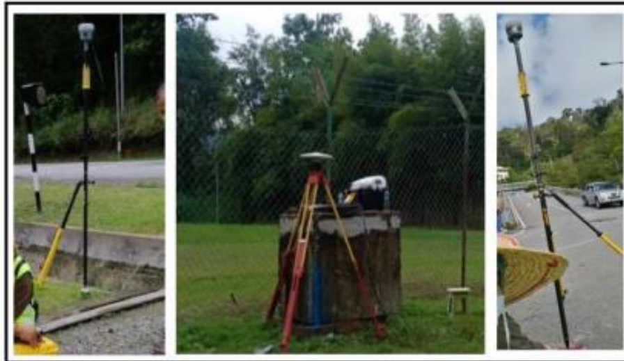
Figure 3. These Are the CORS Malaysia Reference Stations, Bases 1, 2, and 3.
