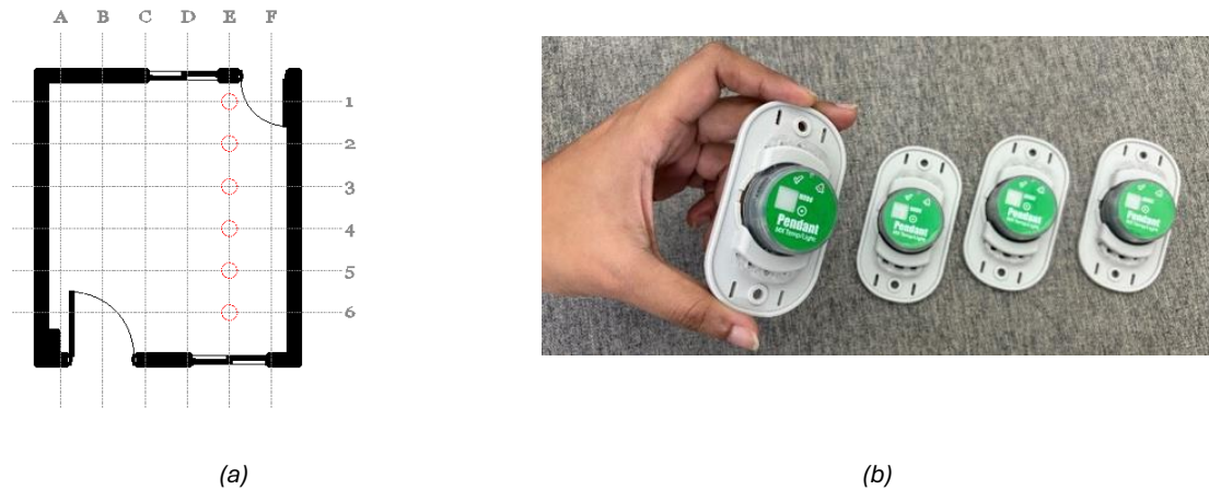
Figure 3. (a) Sensor placements during field measurements; (b) Instrument used for light measurements
